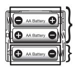
These two batteries power the light and voice alarm function.
