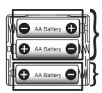
These two batteries power the light and voice alarm
