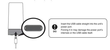
Connect the USB cable's USB connector to a computer or AC adapter, etc., then turn on the power
