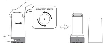
Hold down the base, and pull the tank cap upward to remove it.
