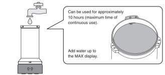
Before adding water, be sure to remove the tank cap from the water supply tank. If water gets on the tank cap, it may cause
