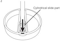
4 Loosen the holder's lock mechanism, then press it into the clip's joint part until a sound is heard to secure the lock.
